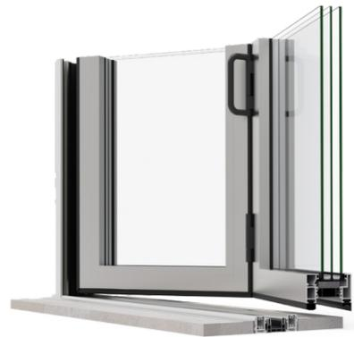
Separate environments and unify spaces with this Bi-fold door system with an 80 mm deep frame. This evolution of the Bi-fold series offers an excellent thermal and acoustic performance, thanks to its 45 mm thermal break and a glazing capacity up to 48 mm.
